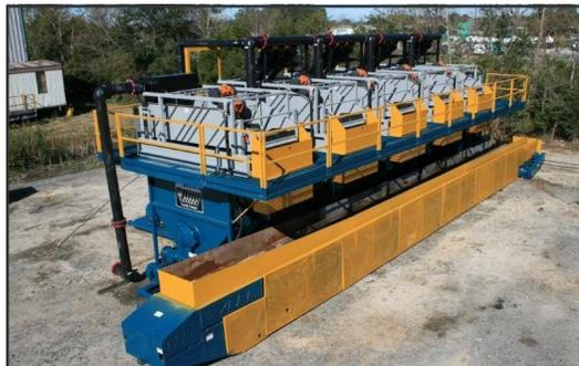
AN ELITE SOLID SEPARATION SYSTEM HIGHLY EFFICIENT IN DEWATERING AND SEPARATING, THROUGH AN ADVANCED COMPILATION OF PUMPS, HYDROCYCLONES, SHAKERS, V-TANKS, TILTED PLATE BAFFLES, AND SHAFTLESS SCREWS.
