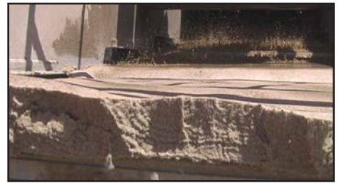
The desander produces a dry product that can be stockpiled immediately.
